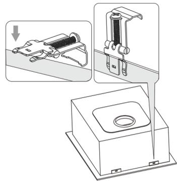
Push the fixing clips onto the cut-outs in the fixing rail to lock them into place.
