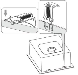
Push the fixing clips onto the cut-outs in the fixing rail to lock them into place.
