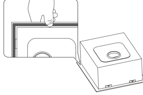
Ensuring the underside of the sink is clean and dry, apply the foam sealing tape around the underside of the sink edge, ensuring it is smooth and without creases or ridges.
