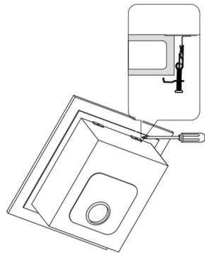
Tighten the fixing clips screws with a hand screwdriver to ensure the sink is secure. Do not over-tighten as this may result in damage.
