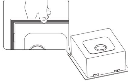
Ensuring the underside of the sink is clean and dry, apply the foam sealing tape around the underside of the sink edge, ensuring it is smooth and without creases or ridges.
