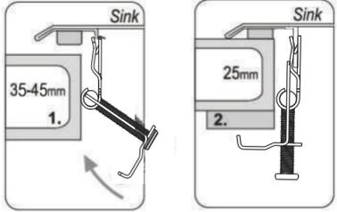
The supplied fixing clips are designed for 35-45mm thick counter tops. If your counter top is thinner, use wood spacers to secure the clips.
